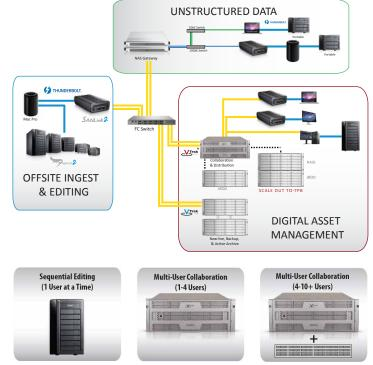
\*Pegasus2: 1 user can write on a file at a time, multiple users can read. VTrak A-Class: Multiple users can write to the same file for true collaboration.
